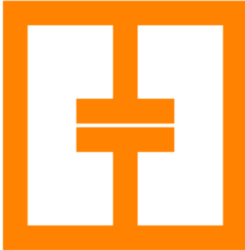
Fig. 1a. Structure and transfer characteristics of a classical eSRR. For the device simulated the sides are 120\ \mu\text{m} , the arms are 10\ \mu\text{m} , and the gap is 2\ \mu\text{m} .
