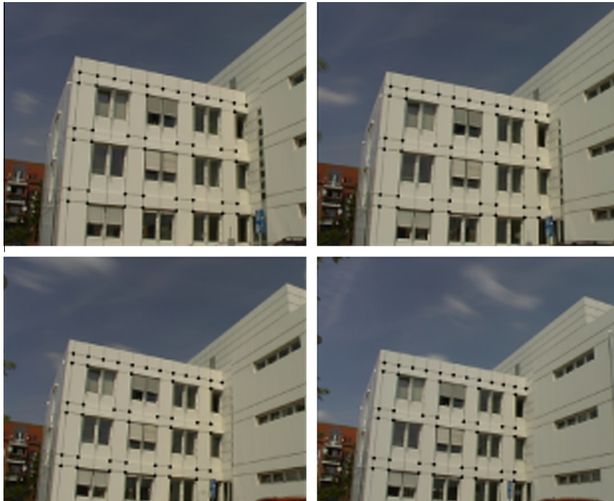
Fig. 7. Real data image sequence: images (numbers 1, 3, 5 and 7) with detected collinear feature points.
