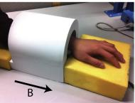
FIG. 1. Magnetostimulation limits were tested in the forearm using a solenoidal coil with 95% homogeneity in a 7 cm-long region. The solenoid created an axial magnetic field (direction shown with the arrow). The measured magnetic field amplitude at the center of the solenoid was 410  $\mu$ T/A.
