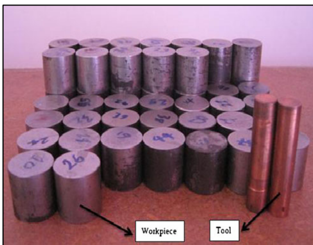
Fig. 13 Workpiece and tool specimens used in ED machining
