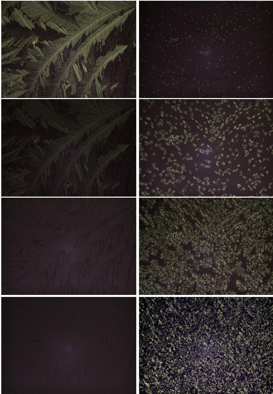
Figure S4. POM imaging during heating (top to bottom, left panel) and cooling (top to bottom, right panel) of \text{CaCl}_2 \cdot x\text{H}_2\text{O} - \text{C}_{12}\text{EO}_{10} with a \text{CaCl}_2/\text{C}_{12}\text{EO}_{10} mole ratio of 2.0.
