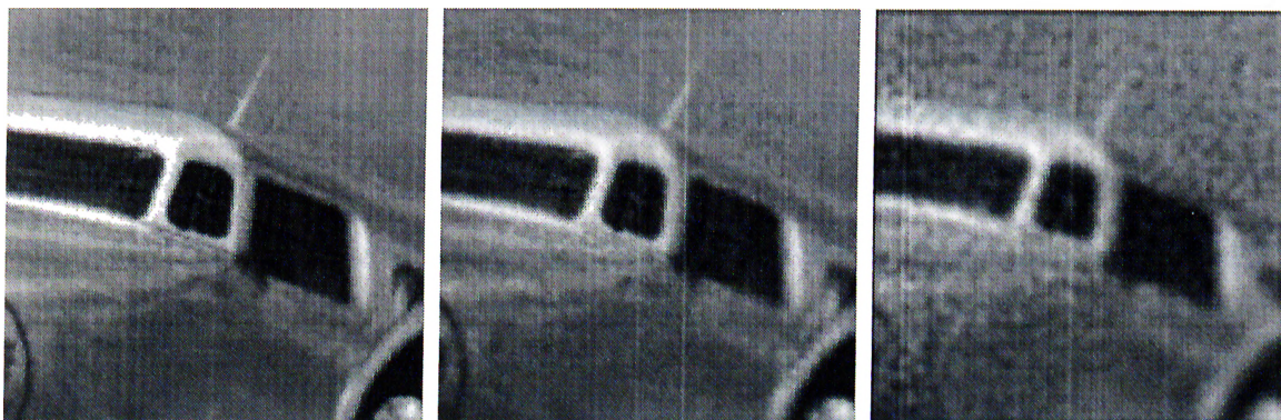
Figure 5.7: Recovered images when the measurement error is (a) 0.2 %; (b) 1 %; (c) 5 %; quoted as a percentage of the mean value of g .
