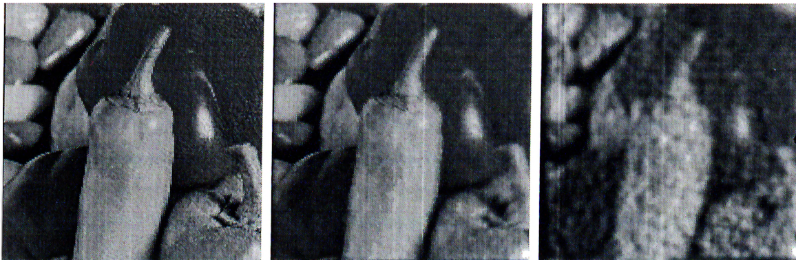
Figure 5.5: Recovered Images for case 2: (a) Without measurement error. (b) With 0.5 % relative measurement error. (c) With 5 % relative measurement error.
