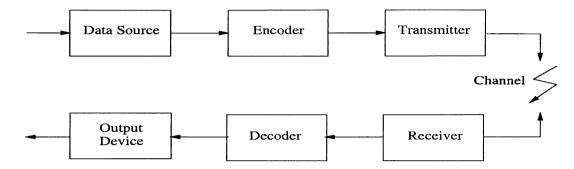
Figure 1.1: A communication system example
