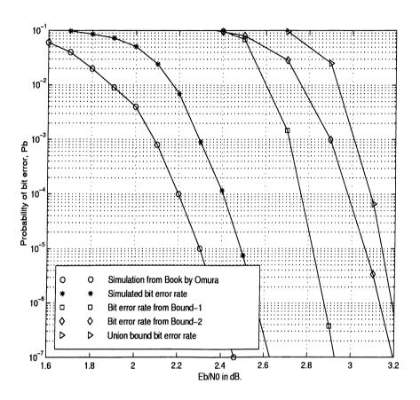
Figure 4.1: Bit error probability of ideally interleaved concatenated system over AWGN channel with soft decision
