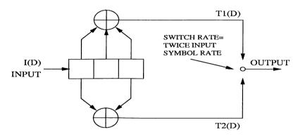
Figure 2.1: Encoder for a R = 1/2, K = 3 convolutional code
