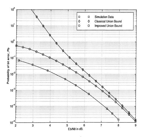
Figure 3.7: Probability of bit error for R = 1/2, K = 3 code over BSC with BPSK modulation
