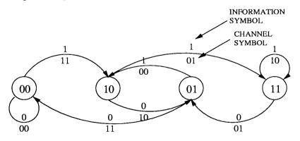
Figure 2.2: State diagram for the R = 1/2, v = 2 convolutional code
