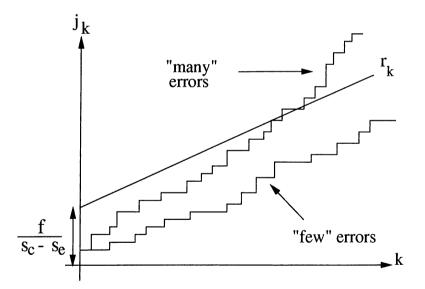
Figure 2.7: Barrier at  $r_k$  which separates paths with many and few errors
