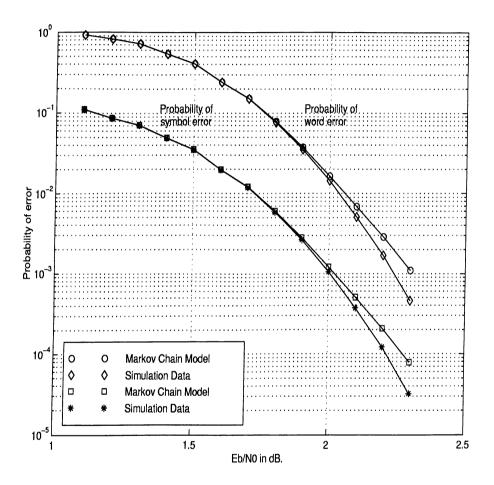
Figure 5.5: Word and symbol error probabilities for non-interleaved concatenated system over AWGN channel and soft decision
