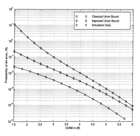
Figure 3.5: Probability of bit error for R = 1/2, K = 3 code over AWGN channel with BPSK modulation
