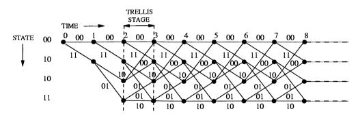
Figure 2.3: Trellis diagram for the R = 1/2, K = 3 convolutional code
