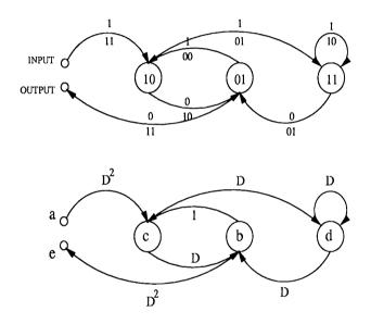
Figure 2.4: State and signal flow diagrams for the R = 1/2, K = 3 convolutional code
