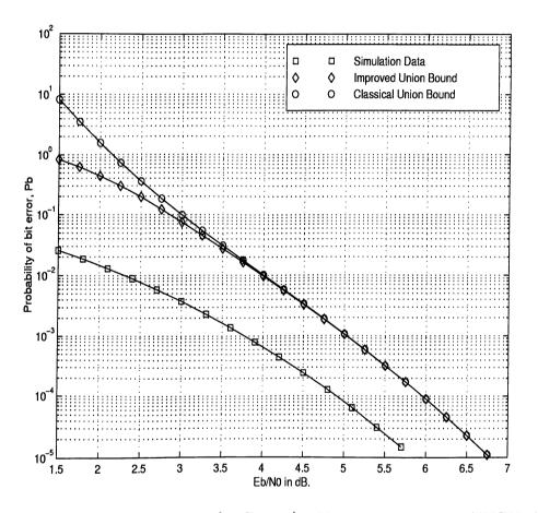
Figure 3.8: Probability of bit error for R = 1/2, K = 3 code over an AWGN channel
