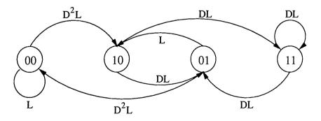
Figure 3.2: State diagram for rate-1/2 constraint-length-3 code
