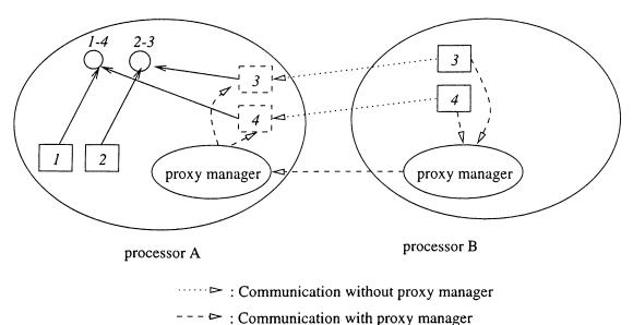
Figure 4.6: Interactions using proxy manager.
