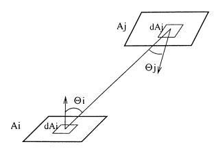
Figure 3.2: Form factor geometry.
