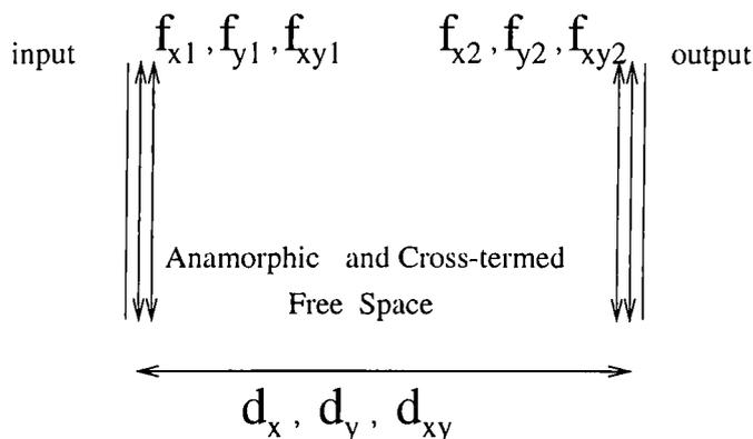
Figure 5.1: Optical set-up that realizes the non-separable fractional Fourier transform
