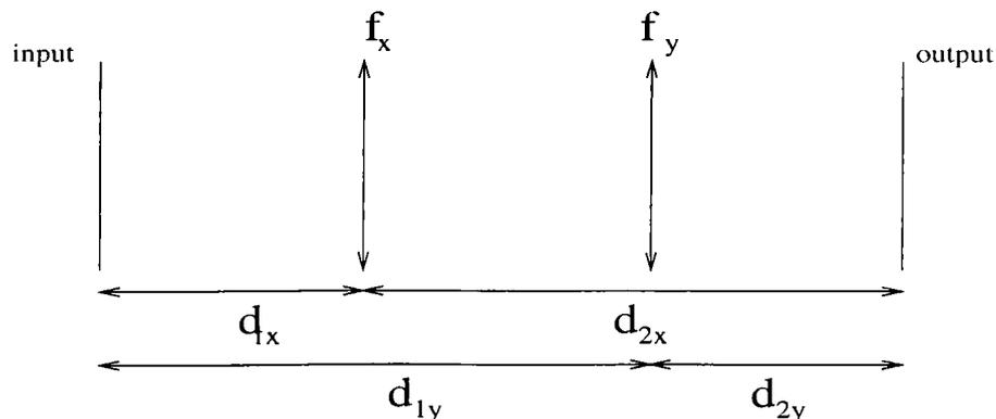
Figure 3.8: Optical set-up with 2 cylindrical lenses and 3 sections of free space
