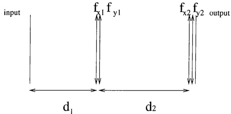
Figure 3.10: Optical set-up with 4 cylindrical lenses and 2 sections of free space
