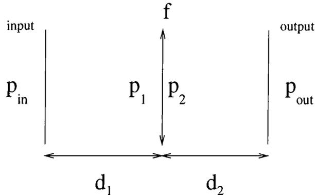
Figure 3.1: Type-1 system that realizes one-dimensional quadratic-phase system
