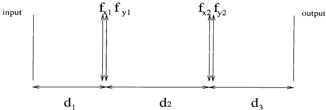
Figure 3.11: Optical set-up with 4 cylindrical lenses and 3 sections of free space
