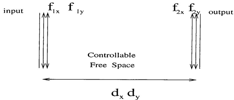
Figure 3.7: Type-2 optical system realizing two-dimensional fractional Fourier transform
