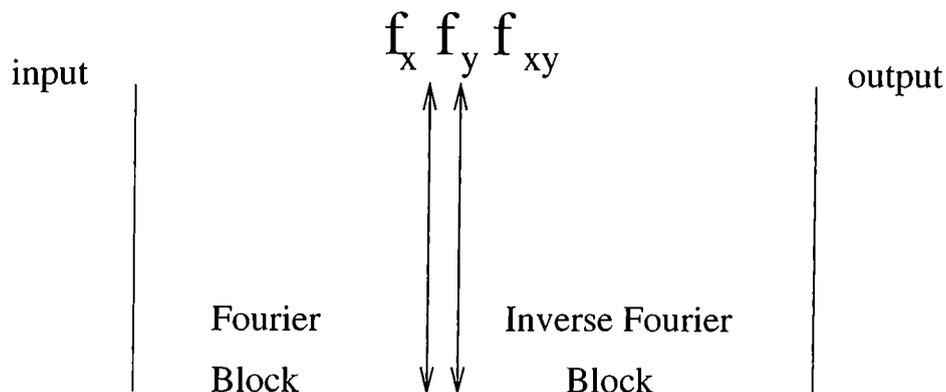
Figure 5.2: Optical set-up that simulates anamorphic free space with cross terms
