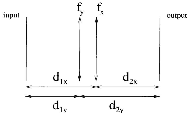
Figure 3.3: Type-1 system that realizes two-dimensional quadratic-phase systems
