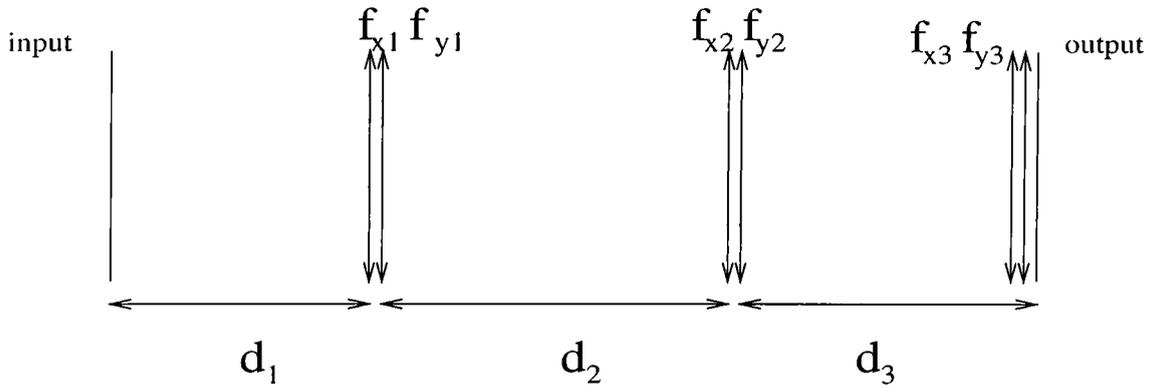
Figure 3.12: Optical system with 6 lenses and 3 sections of free space
