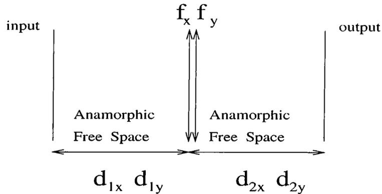
Figure 3.6: Type-1 optical system realizing two-dimensional fractional Fourier transform
