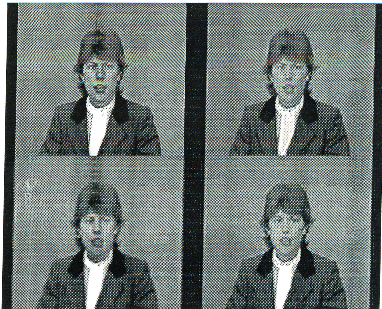
Figure C.1: Filtering results using the decimation filters. In clockwise order starting from upper left: corner: a) original image, the first image in the sequence Claire, b) QCIF/COST, c) NCIF/COST, and d) the unconstrained NCIF design using a 37 \times 37 window, a transition band of 0.17\pi and an attenuation of 50 dB.
