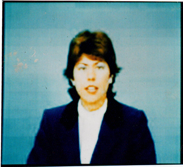
Figure 7.5: Fourth frame of the sequence coded by the COST-SIM2 codec at 16 Kbits/s. (SNR is 33.149 dB for Y comp., 36.533 dB for U comp. and 38.301 dB for V comp.)
