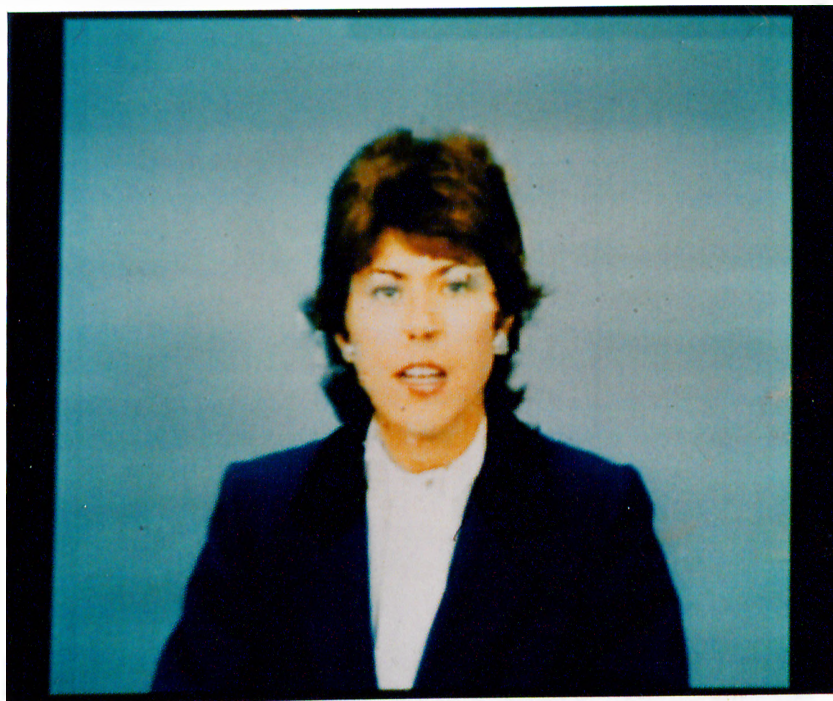
Figure 7.4: Fourth frame of the sequence coded by the non-linear prediction based codec at 16 Kbits/s. (SNRs are 36.124 dB for Y comp., 43.147 dB for U comp. and 46.276 dB for V comp.)
