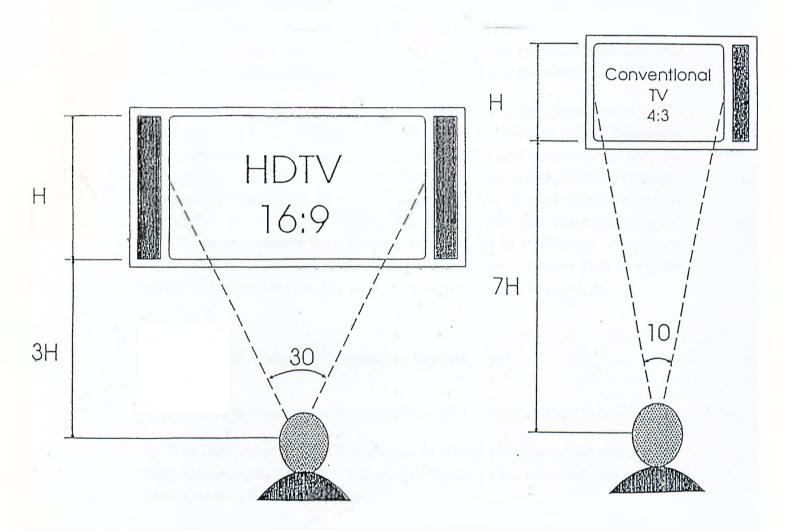
Figure 1.1: Comparison of HDTV and conventional TV
