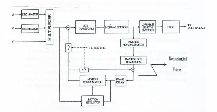
Figure 3.3: Monitoring the reconstructed frame
