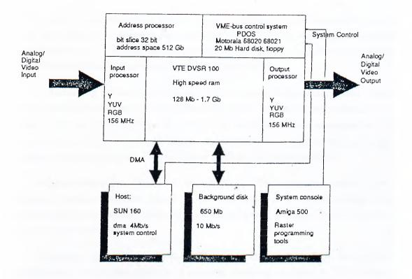
Figure 3.1: The block diagram of the simulation system, DVSR VTE-100
