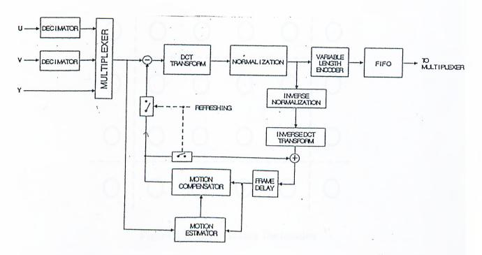
Figure 2.1: Digital Video Encoder block diagram
