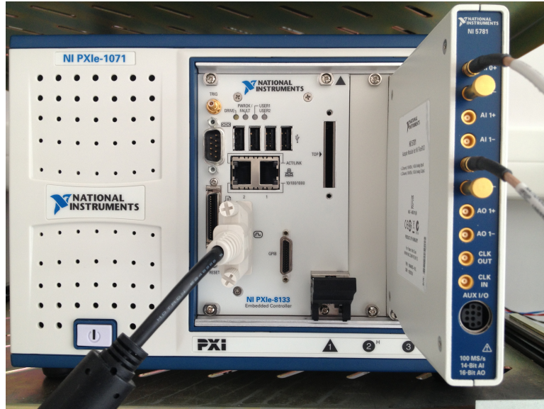
Figure 4.2: PXI system included a chassis, a controller and an FPGA module with a transceiver adapter module.
