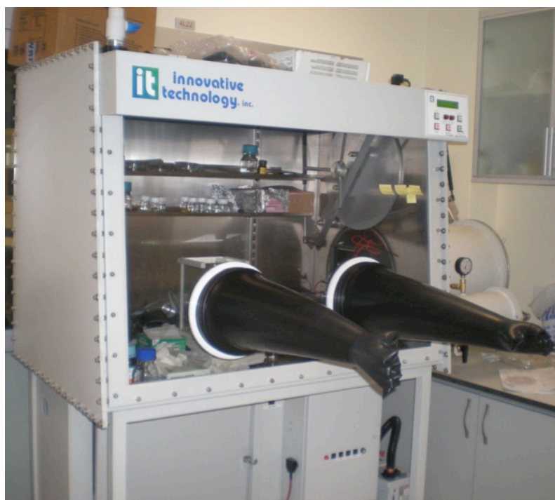
Figure 2.1.2.1.1. Glove box system used for the handling of chemicals that are sensitive to oxygen environment.
