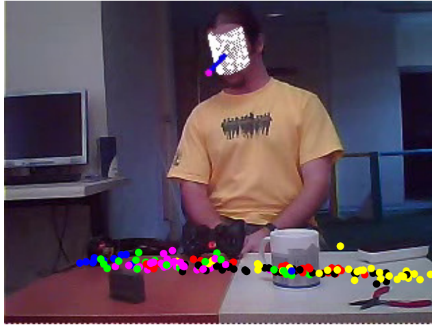
Figure 9.4: Initial estimates for object centers for an exemplary video sequence.
