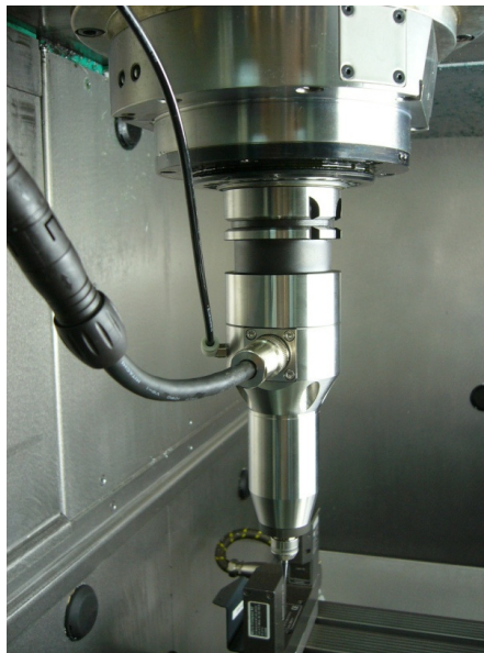
Figure 3.9: Nakanishi HES 510 spindle attached to the machine.
