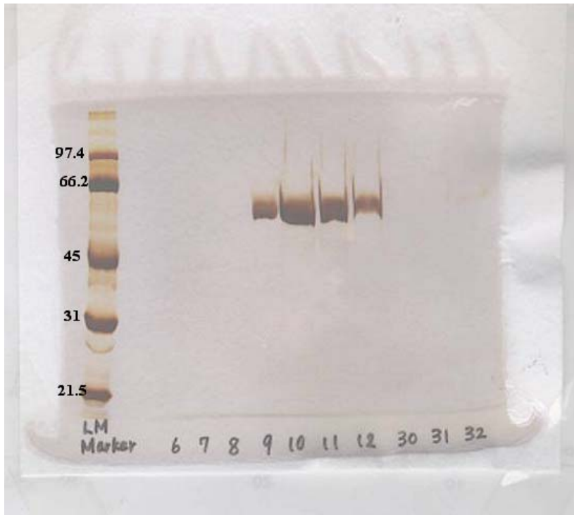
Figure 3.2: Silver-stained gel after SDS-PAGE analysis of elution fractions showing pure protein was isolated with a molecular weight of 55 kDa. The numbers 6~32 show the elution fractions subjected to electrophoresis. LM marker indicates the protein molecular weight marker and the numbers besides each band indicates their corresponding molecular weight in kDa.
