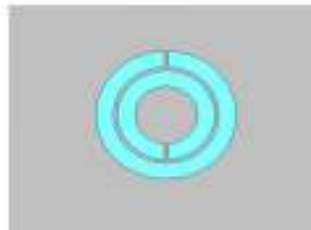
Figure 2.24: Schematic representation of the SRR-shaped aperture model (Gray parts are the metal plate and the blue parts are the gaps).
