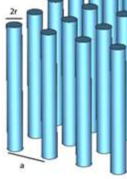
Figure 2.3: The schematic representation of a periodic metallic wire array. a is the lattice constant and r is radius of a single wire.
