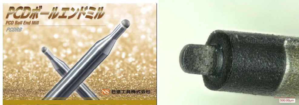
Figure 4.4 (a) A commercial PCD micro tool, (b) PCD micro tool fabricated at Bilkent
