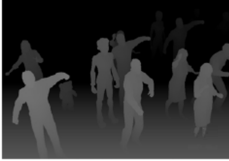
Figure 4.4: A grey-scale output of a sample view rendered by corresponding depth buffer values in pixels
