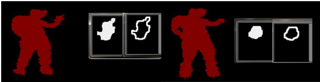
Figure C.2: Images and contours of hand regions from the depth stream. Left: open hand and right: closed hand.
