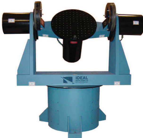
Figure 1.5: An angular position control machine used for inertial sensor calibration [5].
