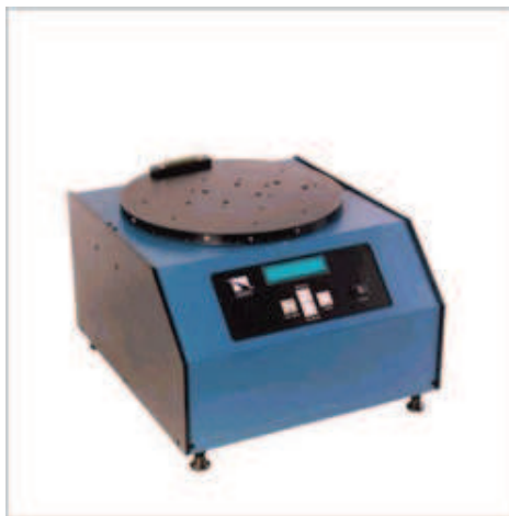
Figure 1.7: A rate table used for gyroscope calibration [7].
