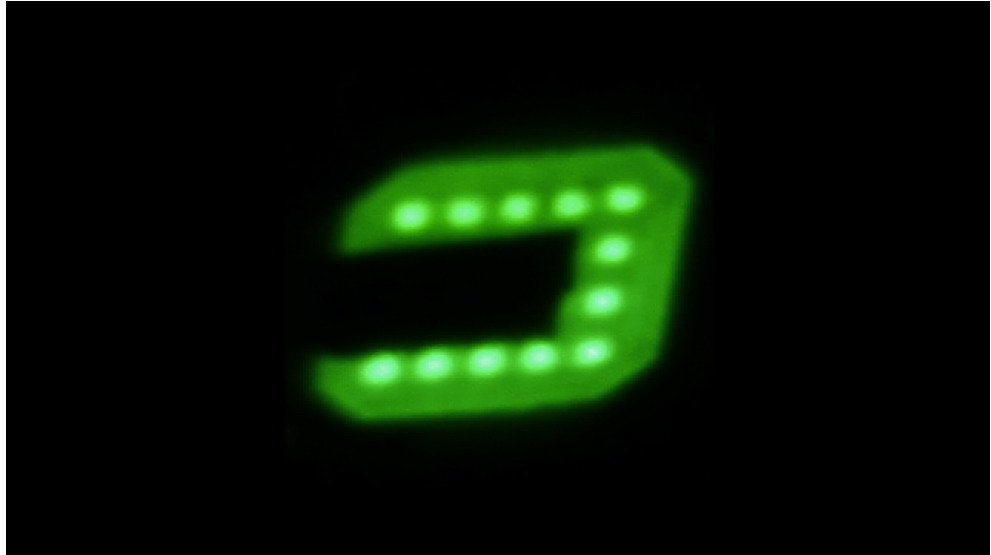
Figure 3.6: An image of the LED array on the object plane: the object is first imaged onto this plane by a projector lens to control both the depth and the size of the object. (Reprinted from “Integral imaging using phase-only LCoS spatial light modulators as Fresnel lenslet arrays,” Ali Özgür Yöntem and L. Onural, J. Opt. Soc. Am. A vol. 28, no. 11, pp.2359-2375, 2011. ©2011 OSA.)
