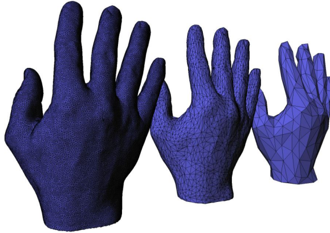
Figure 2.1: A mesh (leftmost) and two levels of simplification results using a popular mesh modification library (CGAL)
