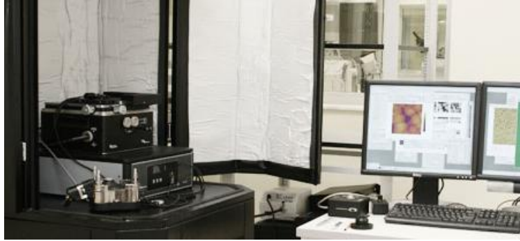
Figure 3.12: Asylum Research MFP-3D AFM used for the morphological characterization of \text{Ga}_2\text{O}_3 thin films.
