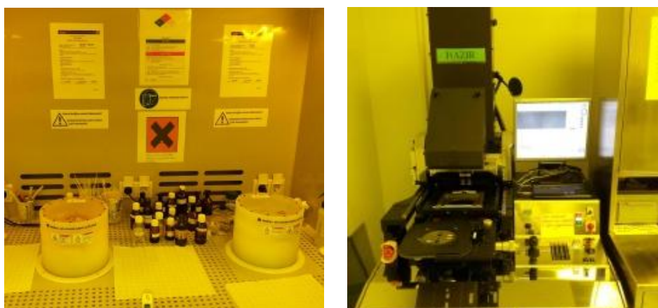
Figure 3.7: (a) Hexametyldisilazane and AZ5214E photoresist were spin coated on top of the samples by using Laurell spinner system. (b) Electronic Vision Group EVG620 Mask Aligner used for the alignment and exposure of photoresist coated samples.
