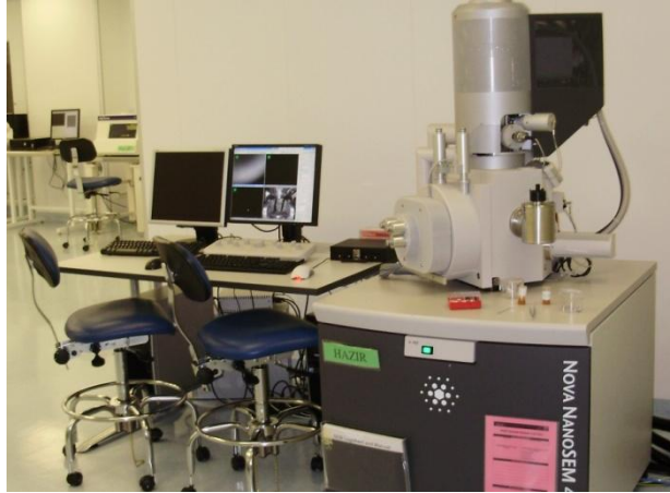
Figure 3.11: Nova NanoSEM scanning electron Microscope used for the surface imaging of \text{Ga}_2\text{O}_3 thin films and \text{HfO}_2 nanostructures.
