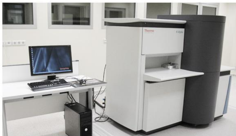
Figure 3.13: Thermo Scientific K-Alpha X-Ray photoelectron spectroscopy system located at UNAM Characterization Laboratories.
