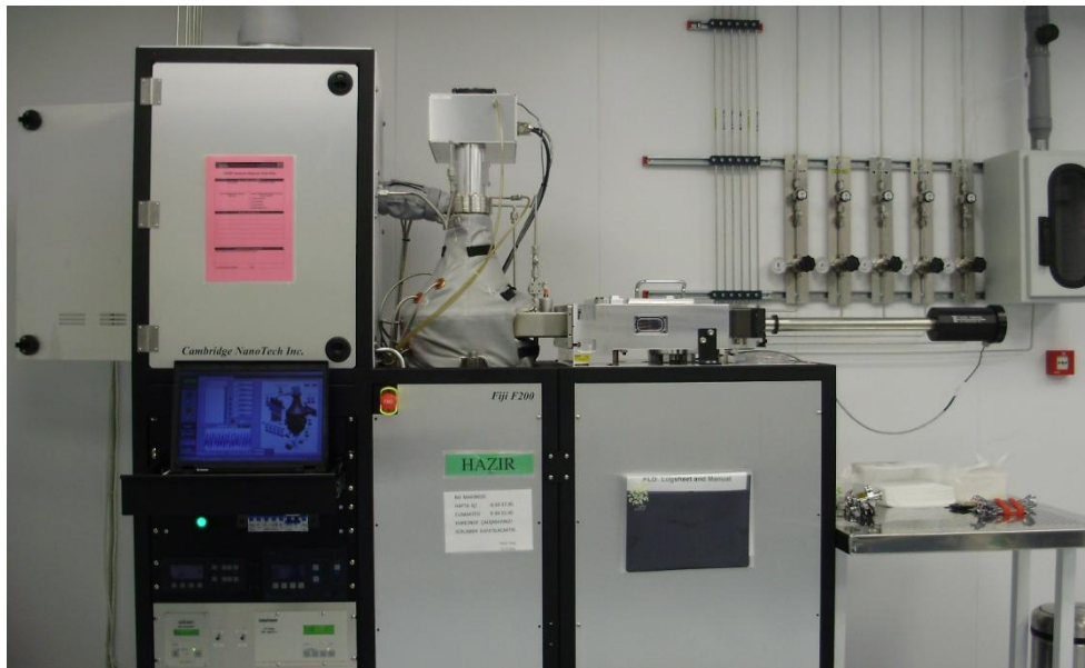
Figure 3.1: Fiji F200 LL plasma-enhanced atomic layer deposition system, which was used for the \text{Ga}_2\text{O}_3 depositions.
