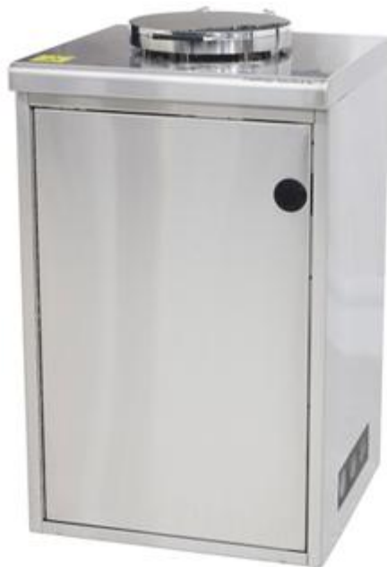
Figure 3.10: Savannah S100 thermal ALD reactor (Cambridge Nanotech Inc.) used for the deposition of HfO 2 on electrospun nylon nanofibers.
