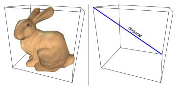
Figure 3.2: Left: Axis-aligned bounding box; right: diagonal of the axis-aligned bounding box.
