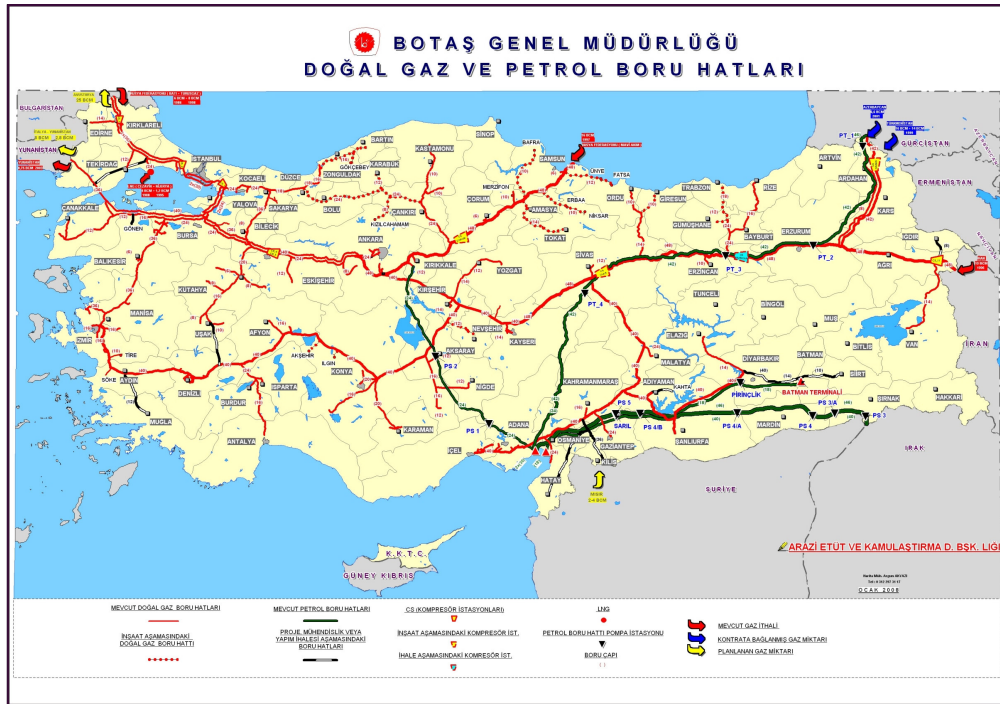
Turkey's Existing Pipeline System
