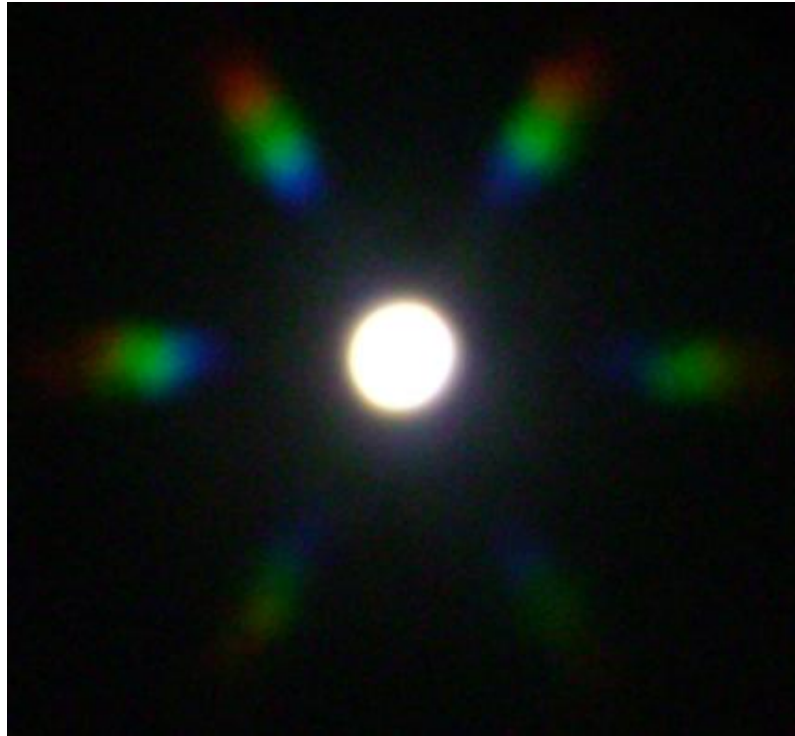
Figure 4.32: Transmission mode diffraction photograph of photonic crystals.
