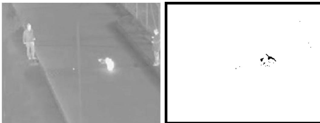
Figure 3.3: Results of Dynamic Background Subtraction and Morphological Opening using a disk of a radius 2 pixels.
