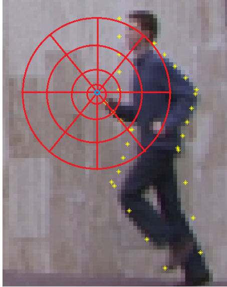
Figure 3.2: This figure demonstrates the shape context calculation process. In shape context, a circular grid is positioned over the sample points of an image and a histogram SC with size r \times u is generated for each point where r is the number of radial bins and u is the number of orientation bins.
