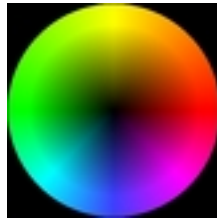
Figure 4.6: Optical flow vector color codes. Direction of the flow is coded with colors, and the magnitude is coded with intensities.
