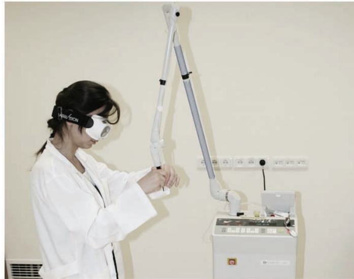
Figure 4.1: Lumenis C40 CO 2 laser system for medical application which is to be embedded with a laser beam coupling system.
