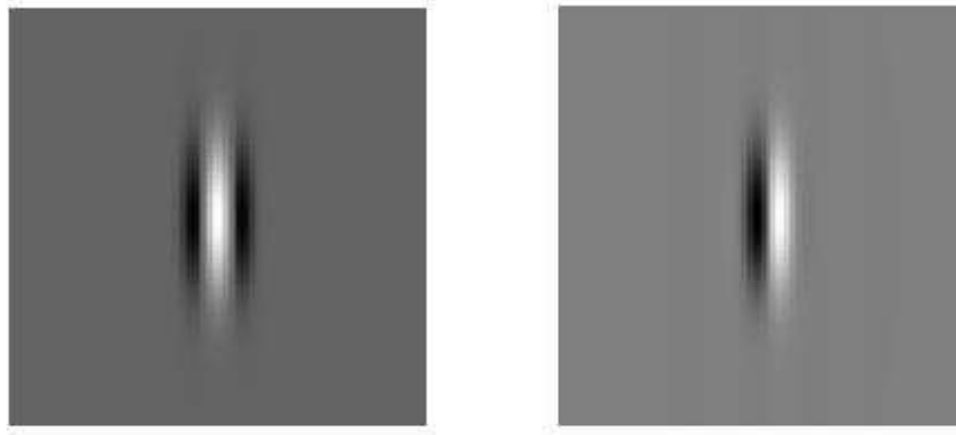
Figure 2.6: Intensity plot of the real (left) and imaginary (right) parts of a vertically oriented 2-D Gabor filter in spatial domain with mid-gray values representing zero, darker values representing negative numbers and lighter values representing positive numbers.
