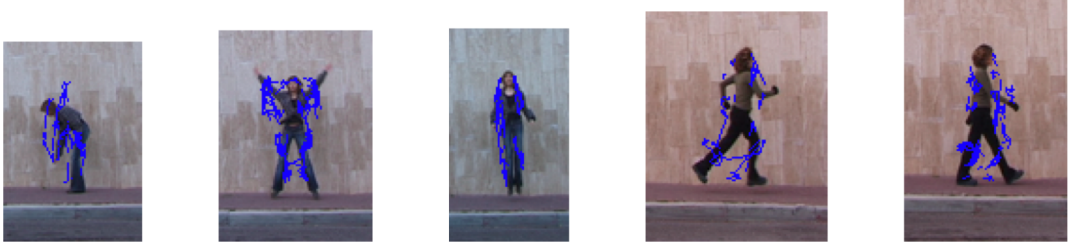
Figure 3.9: This figure illustrates the global line-flow of different actions ( from left to the right ): bend, jumping jack, jump in place, running and walking. Notice that the line-flow vectors are in different orientations in different spatial locations so that ‘bend’, ‘jumping jack’ and ‘jump in place’ can be easily distinguished. Although, the global line-flow of ‘running’ and ‘walking’ seem similar, notice the difference in the density of the lines. Sparser lines represent faster motion, whereas dense lines represent actions with slower motion.
