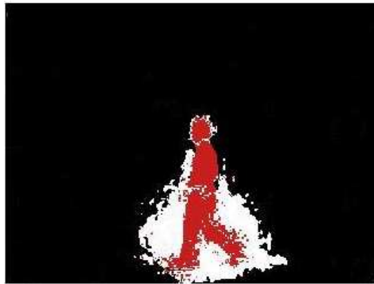
(b) Detected moving object (shaded in red) and shadow regions (dark shaded)
