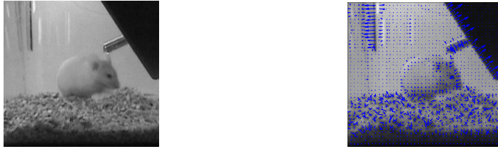
(a) Original real world image. (b) Gradient vectors overlaid on original image.
