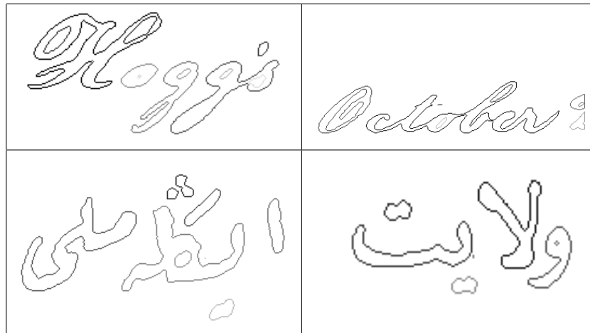
Figure 3.3: The contour segments extracted from the binarized images for word spotting task.
