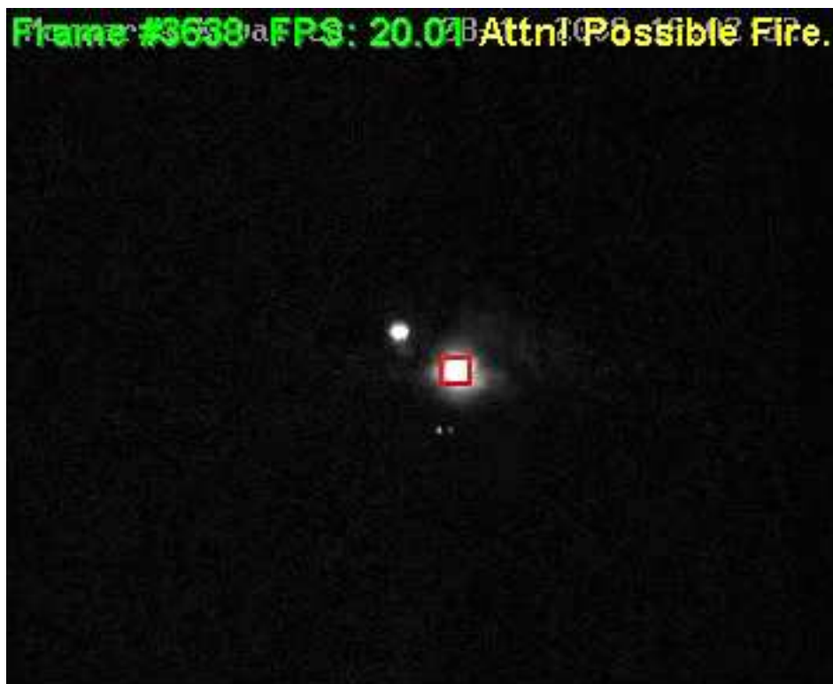
Figure 3.5: Correct alarm for a fire at night and elimination of fire-truck headlights.
