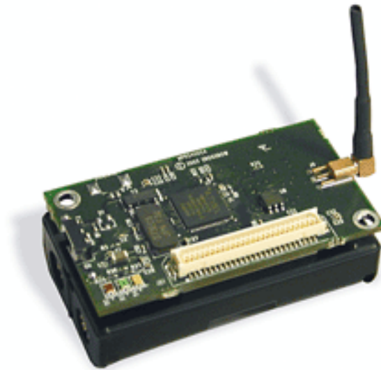
Figure 2.1: MicaZ sensor node
