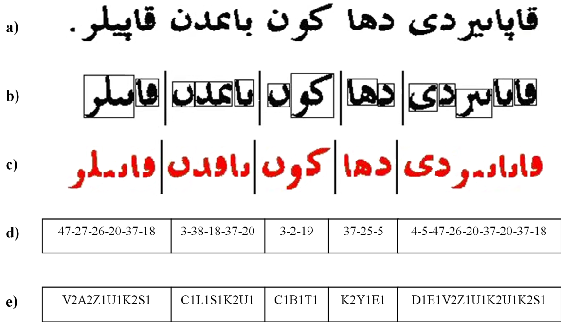
Figure 5.1: Grouping recognized letters into words and mapping these words into ASCII characters.
