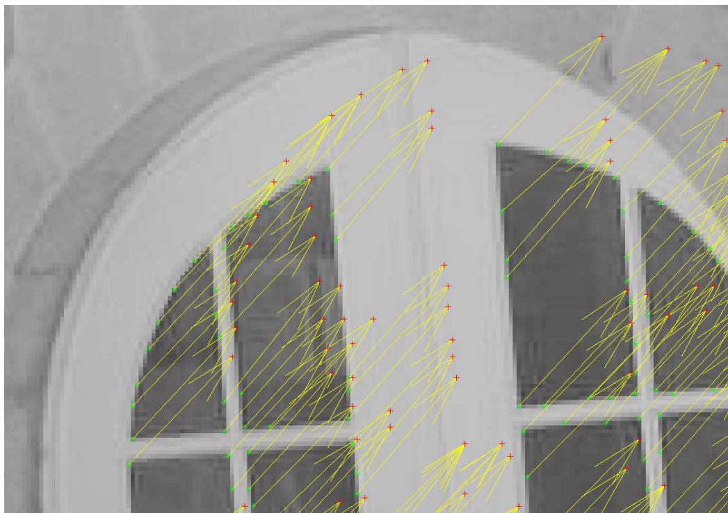
Figure A.2: The matched feature points among points detected shown in Figure A.1 by using gray-level patch description. The original “bike” image couple is taken from Oxford University Visual Geometry Group.
