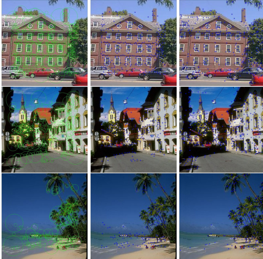
Figure 3.7: Results of two keypoint detectors. First column shows Kadir-Brady keypoint results with scale circles. Second column shows the Kadir-Brady keypoint coordinates while the third column shows SIFT detector keypoint coordinates.
