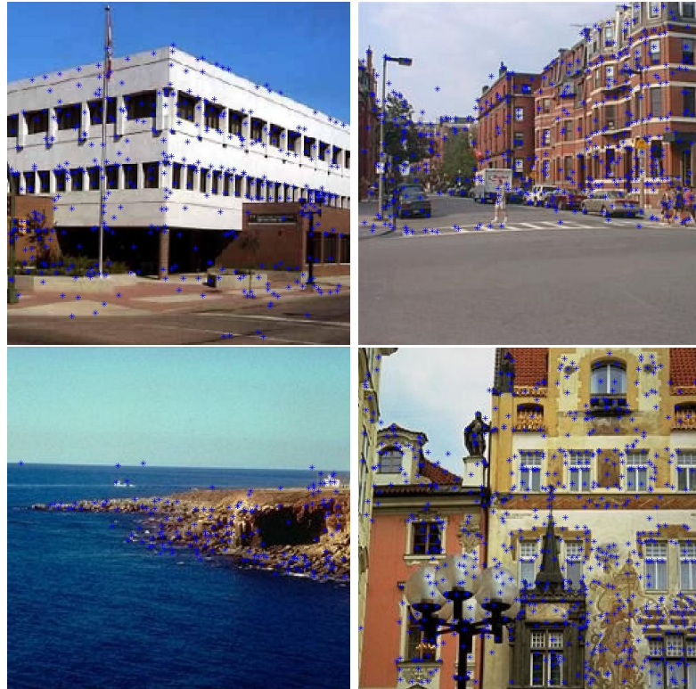
Figure 3.3: Results of keypoint detector.
