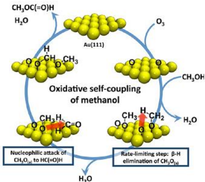
Figure 6. Mechanism for the self-coupling of methanol on O/Au(111). (Permission requested for reproduction from Ref 88).
