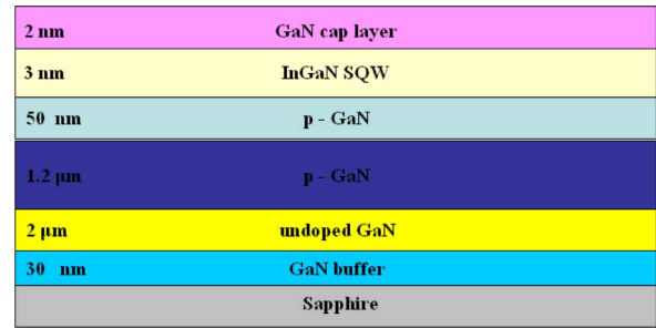
Fig. 8. Epitaxial structure of our wafer for energy transfer from single QW (SQW) to colloidal NCs for yellow/green emission.
