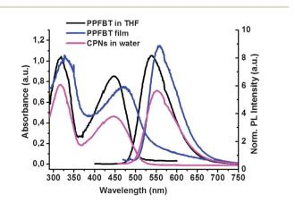
Fig. 2 UV-vis absorption and emission spectra of PPFBT in THF ( $\lambda_{exc}$  = 447 nm) and as a film ( $\lambda_{exc.}$  = 472 nm), and of a dispersion of the nanoparticles in water ( $\lambda_{exc.} = 447$  nm).
