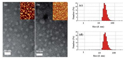
Fig. 5 TEM images of CPNs (a) and CPT-loaded CPNs (b); the insets are their AFM images (scale:  $0.5 \times 0.5 \mu m$ ). Dynamic light scattering histograms of CPNs (c) and CPT-loaded CPNs (d).
