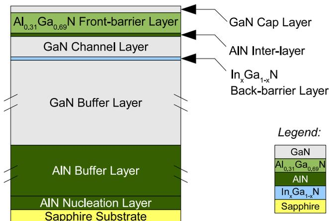
Fig. 1. The layer structure of the studied samples.
