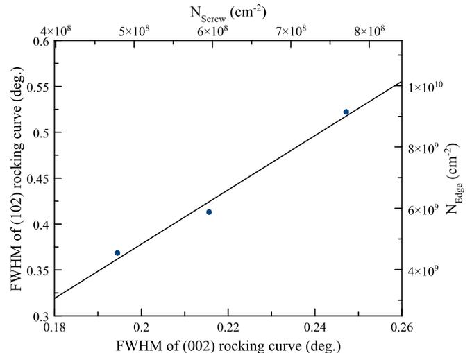
Fig. 5. FWHM values of the (102) rocking curve versus (002) rocking curve for the sample with  $\text{In}_x\text{Ga}_{1-x}\text{N}$  back-barriers with different In mole fractions. Line is a linear fit.
