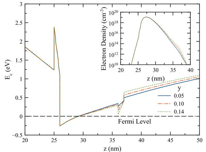
Fig. 2. Conduction band profile for the studied samples where  $y = 0.05$  (blue full line),  $y = 0.10$  (red dash-dots),  $y = 0.14$  (green dots) and Fermi level (black dashes) Inset: electron density probability distribution in pseudotriangular quantum well formed near the AlN inter-layer and at the GaN channel layer. (For interpretation of the references to color in this figure legend, the reader is referred to the web version of this article.)
