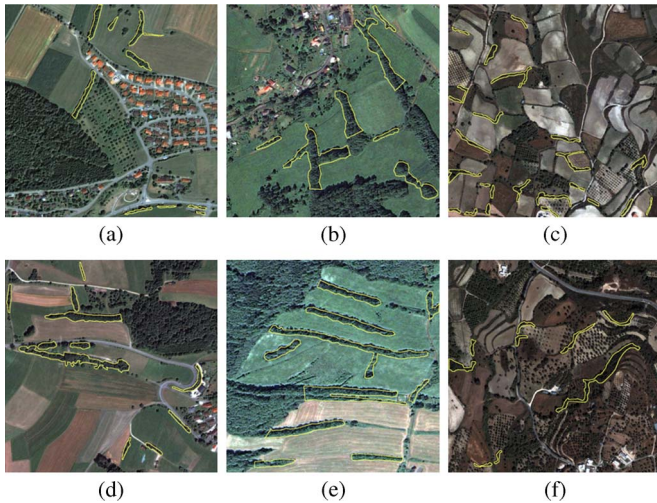
Fig. 1. Example QuickBird images (pan-sharpened visible bands) containing linear strips of woody vegetation marked with a yellow boundary by an expert. Linearity of their shape and woodyness of their texture distinguish these structures from the rest of the image. Linearity is defined here as a piecewise elongation along the major axis while having an approximately constant width, not necessarily in the strict sense of a perfectly straight line. Woody vegetation consists of trees and bushes. Note that other linear but nonwoody structures and woody vegetation areas that are not linear are not marked. (Raster images in this paper are 1000 \times 1000 pixels in size corresponding to 600 \times 600 m.) (a) Germany. (b) Czech Republic. (c) Cyprus. (d) Germany. (e) Czech Republic. (f) Cyprus.
