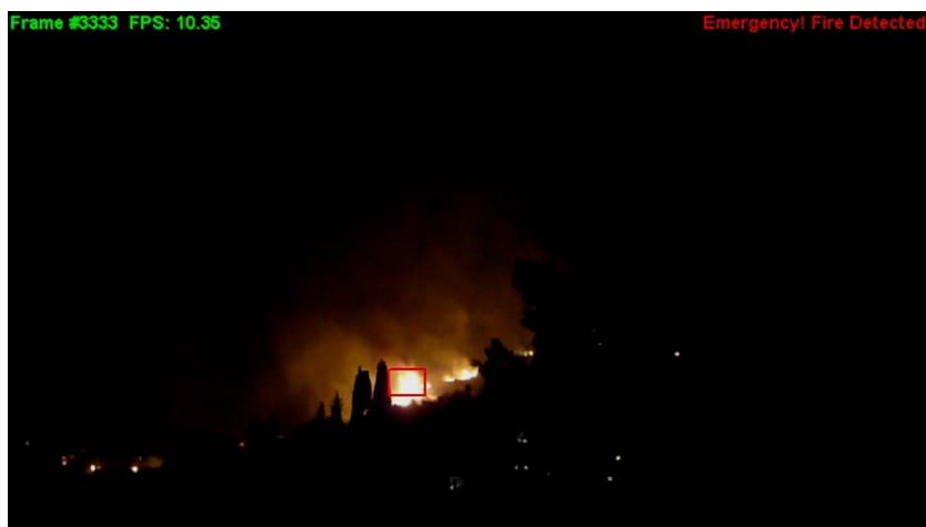
Fig. 8. Detection results on an actual forest fire at night.
