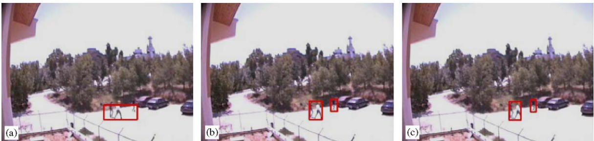
Fig. 4. Detection results for (a) subband domain, (b) VSAM and (c) GMM based methods in a parking lot sequence recorded in the day-time.
