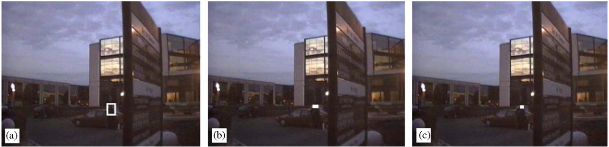
Fig. 5. Detection results for (a) subband domain, (b) VSAM and (c) GMM based methods in a parking lot sequence recorded at night.
