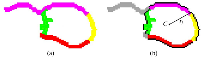
Fig. 7. Determining the outermost pixels and calculating a radial distance r_i . The primitive segments on the correct sides of other primitives are identified and the outermost pixels are selected. Nonselected primitive segments are indicated in gray.
